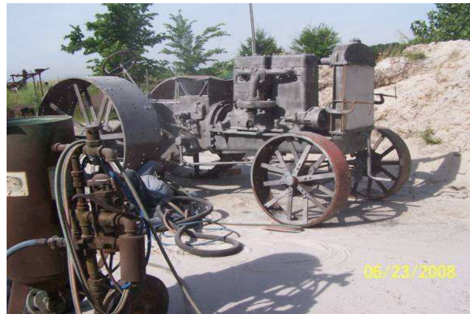
Bill Montgomery - sand blasting for a new finish.
